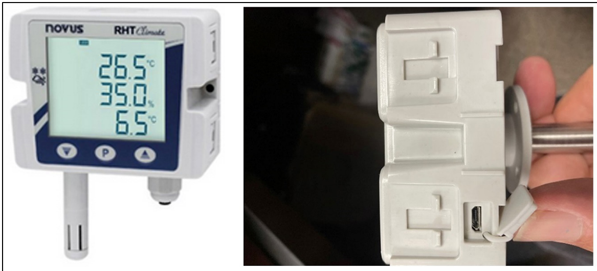
Figure 19—NOVUS RHT climate instrument: Left, basic display; Right, side view with clips that open and the USB programming port.
