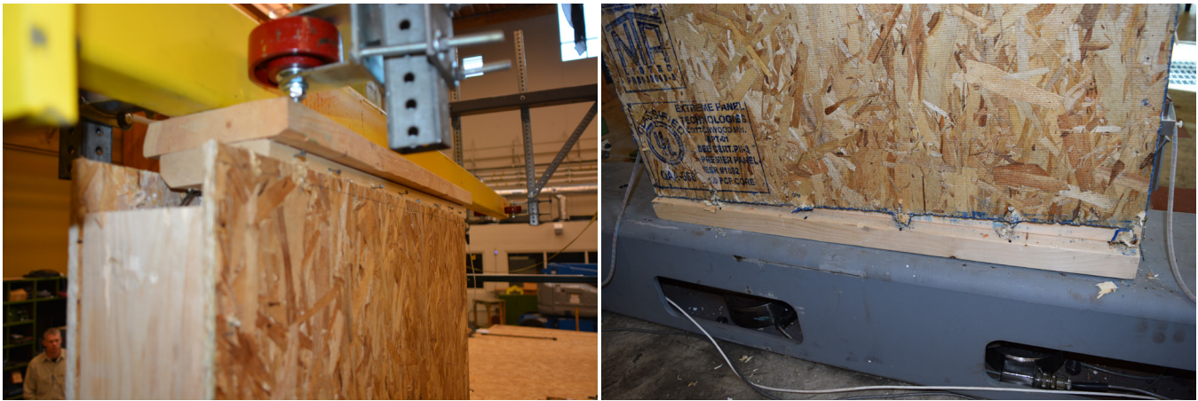
Figure 9. Failure modes for single-panel SIP tests.
