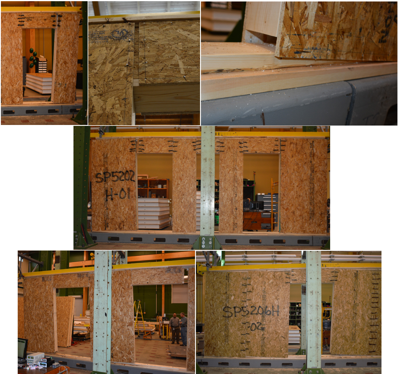
Figure 11. Failure modes for multiple-panel SIP walls with openings.
