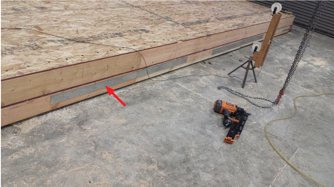
Figure 8. Chord strap from Simpson Strong-Tie CMSTC16 coil straps cut to 6-ft lengths for use in Part B SIP diaphragm tests.
