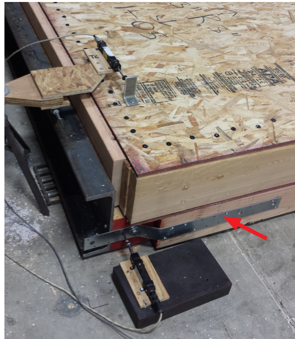
Figure 9. Framing anchor (Simpson Strong-Tie MST126) used in Part B SIP diaphragm tests.
